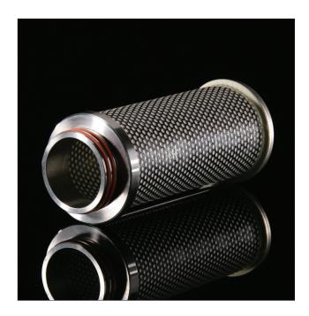
BIO-X II air sterilization filter cartridges utilize a borosilicate microfibre media. This media has proven to be particularly effective in the removal of sub-micron particles as small as 0.01 micron, therefore ensuring the removal of all microorganisms, including bacteria and viruses.
